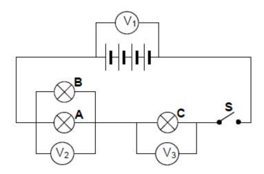
9.1 Calculate the effective resistance of bulbs **A** and **B**. (3)
