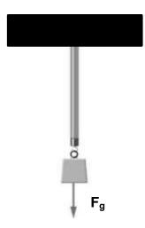
A bungee cord with a length of 0,75 m and diameter of 20 mm was used during the experiment. A mass piece of 20 kg was hung from the end of the bungee cord. The cord elongated by 50%.
