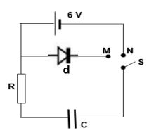
Switch **S** is initially at position N, charging the capacitor.
